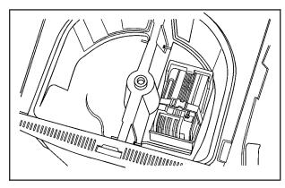
2. Locate the tire inflator kit on the driver's side of the vehicle, near the back corner of the trunk.
